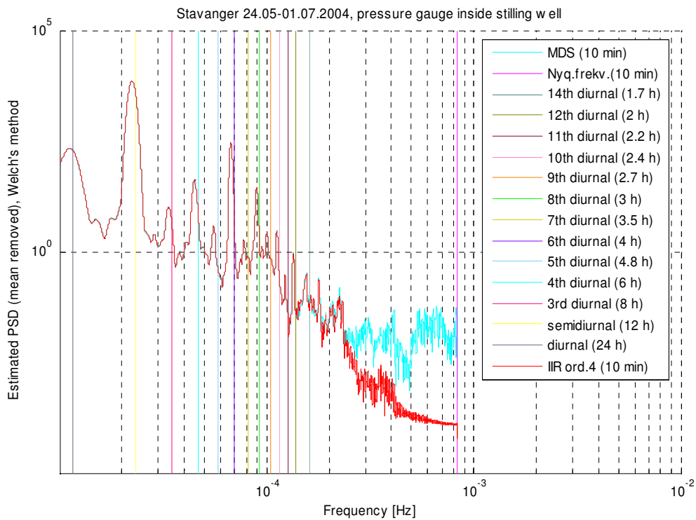
Figure 8-15 Estimated PSD of water level data (pressure gauge inside a stilling well filtered and decimated and MDS).
